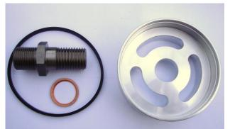
There is (usually) a small grub screw which retains the boss and this must be unscrewed first. Access to the grub screw is gained through a hole in the casting at 90° to the boss. Remove the grub screw and then remove the boss by unscrewing it with tommy-bar through the large centre hole. Remove the splash plate (the large steel 'washer').
